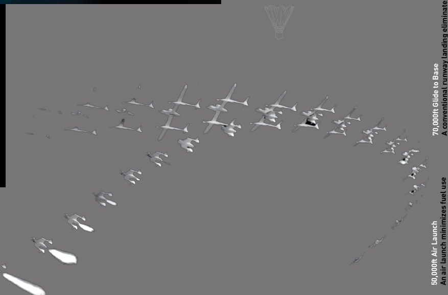
50,000ft Air Launch: An air launch minimizes fuel use and increases safety.
